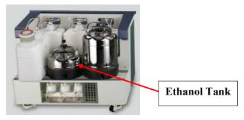
4.3. On the main toolbar select Cytometer > Fluidics Shutdown and follow the software prompts. The final step cleans the flow cell with Shutdown Solution.
