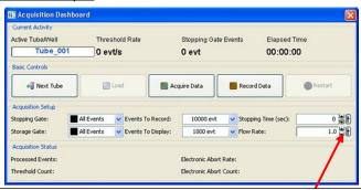
Adjust the flow rate by pressing the small arrow
