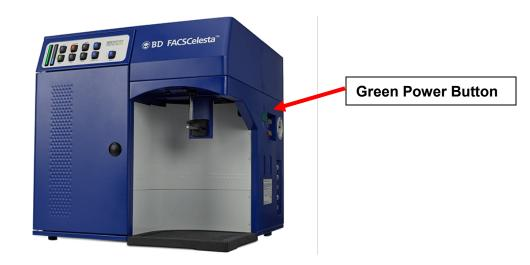
1.4. Ensure that there is a tube with approximately 2 ml of diH<sub>2</sub>O on the SIP. Press the PRIME button to prime the instrument. Repeat priming again after the instrument has returned to STANDBY.
